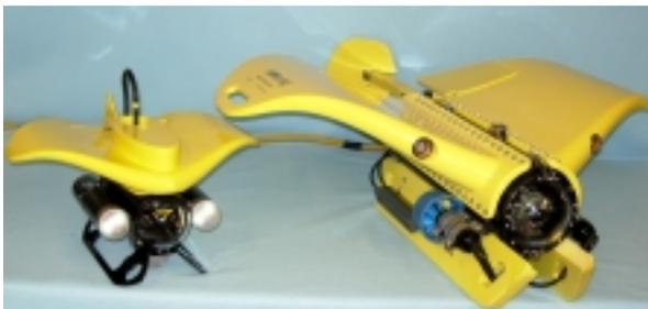
MicroWing™, designed for VideoRay® micro-ROVs, is the newest addition to the Nova Ray, Inc. family of products, using the Nova Ray® arcuate wing technology.
