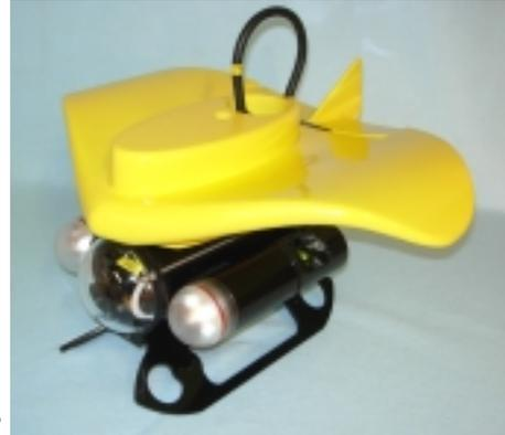
Adding the removable MicroWing™ system makes it easy to tow the VideoRay® micro-ROV, and provides more underwater capabilities.
